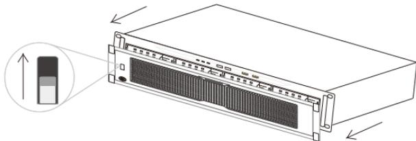
3. Press the button on the front panel of a hard disk tray until the cover on the front panel pops open.
